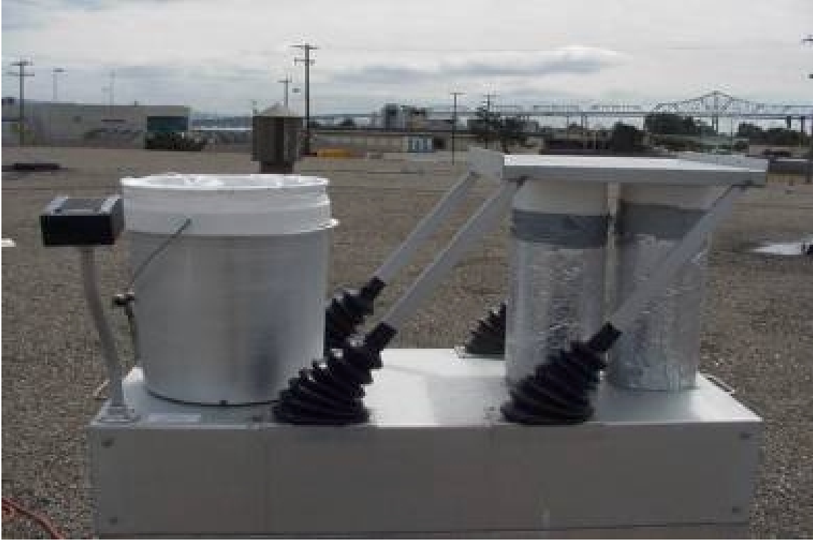
Figure 2. Wet Deposition Sampler (Aerochem Metrics)
