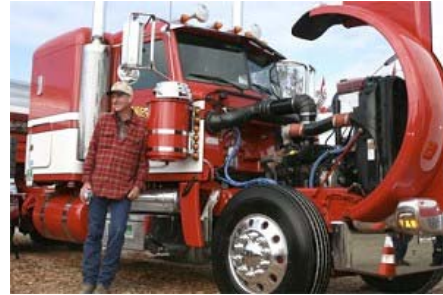
Rob Hilarides of Hilarides Dairy in Lindsay, Calif., listens to the engine of his truck, which was converted from diesel to run on biomethane, on Wednesday, Feb. 11, at the World Ag Expo in Tulare, Calif. The biomethane gas was produced from dairy waste at his farm. Photo by Cecilia Parsons/Capital Press
