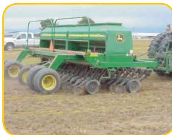
Figure 2. John Deere 1590 No-Till drill that Tom uses. Down pressure and a slower speed is critical for seed placement into soil.
